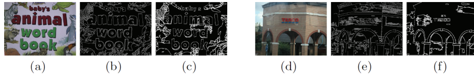
Fig. 2. Illustration of the gradient-based edge image (b)(e) and the smoothness-based edge image (c)(f) for the left sample image (a) with shadows and the right one (d) with low contrast. Note that the smoothness-based edge image better depicts the text contour than the gradient-based one.
