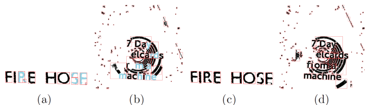
Fig. 5. Results of the original CC algorithm (left) on sample image with intra-character confusions (a) and sample image with inter-character confusions (b), and our edge-augmented CC algorithm (right) on the same sample images (c) and (d). Note that CCs colored in blue are false extraction results by the original algorithm.
