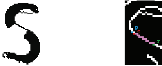
Fig. 6. Illustration of the proposed edge-augmented CC algorithm. Left is the SWT image with the intra-character error as the input of the algorithm. Right is the edge image, in which pixels in pink color correspond to the traversing path of the algorithm connecting the ES pixels p and r on the fragmented contour of the character.
